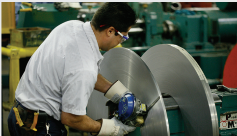
coils being banded on turnstyle
