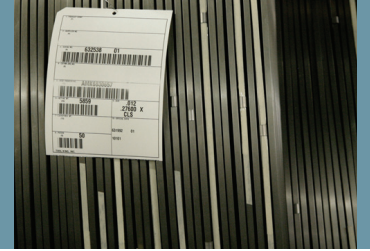
.012" x 0.276" cold rolled awaiting oscillate winding
