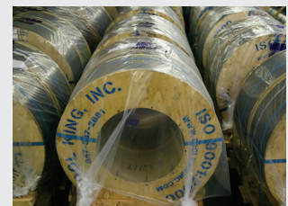
oscillate wound coil on spools with plastic shrouding
