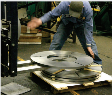
positioning slit coil on skid
