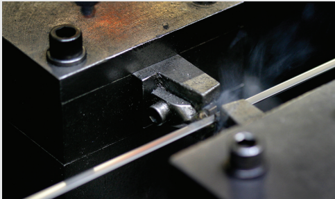
cold rolled being square edged
