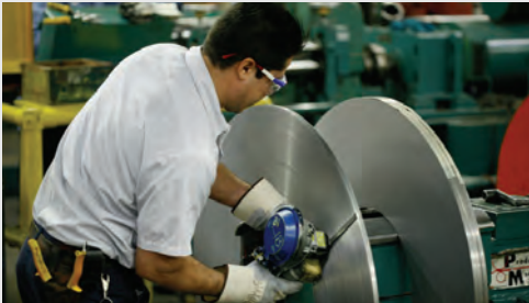
coils being banded on turnstyle
