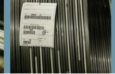
.012" x 0.276" cold rolled awaiting oscillate winding
